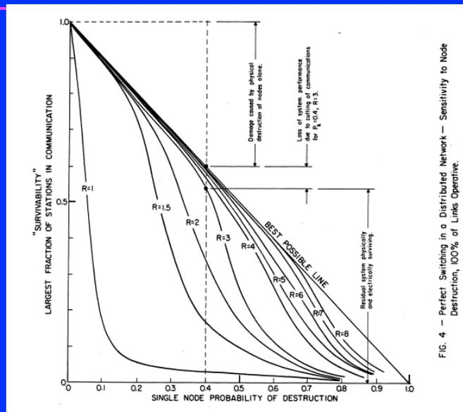
FIG. 4 - Perfect Switching in a Distributed Network - Sensitivity to Node Destruction, 100% of Links Operative.
