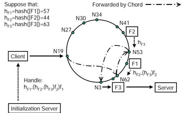
**Figure 8. ANON with Chord as the underlying transport network, i.e., ANON over Chord. In contrast, nested encryption is now applied to Chord IDs instead of IP addresses. The IP address of a forwarder is used by a hash function to derive its Chord ID; Chord nodes will forward packets addressed to a forwarder as if it were a request for the object with the same Chord ID.**
