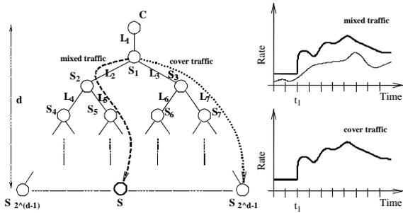
**Figure 3. The cover-traffic tree for our model problem of Section 6.1. C is the client and S is the target server. The diagram on the left illustrates that the total traffic on the path from C and S is the sum of real and cover traffic, while that on any other link is just the cover traffic. The two diagrams on the right indicate that at any given time the total traffic over any link looks the same with or without real traffic.**
